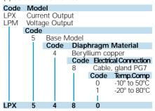
(2) State minimum and maximum pressure and corresponding output signal. (3) State options (if required)
