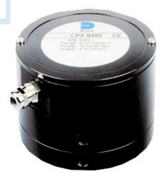
The LP 5000 series accurately measure low differential or relative pressure of gases and liquids from 0.5mbar to 10 bar full scale. With a choice of current or voltage output, they are suitable for uni-directional (e.g. 0 to 20mbar) or bi-directional (e.g. -20 to 20mbar) pressure measurements.
